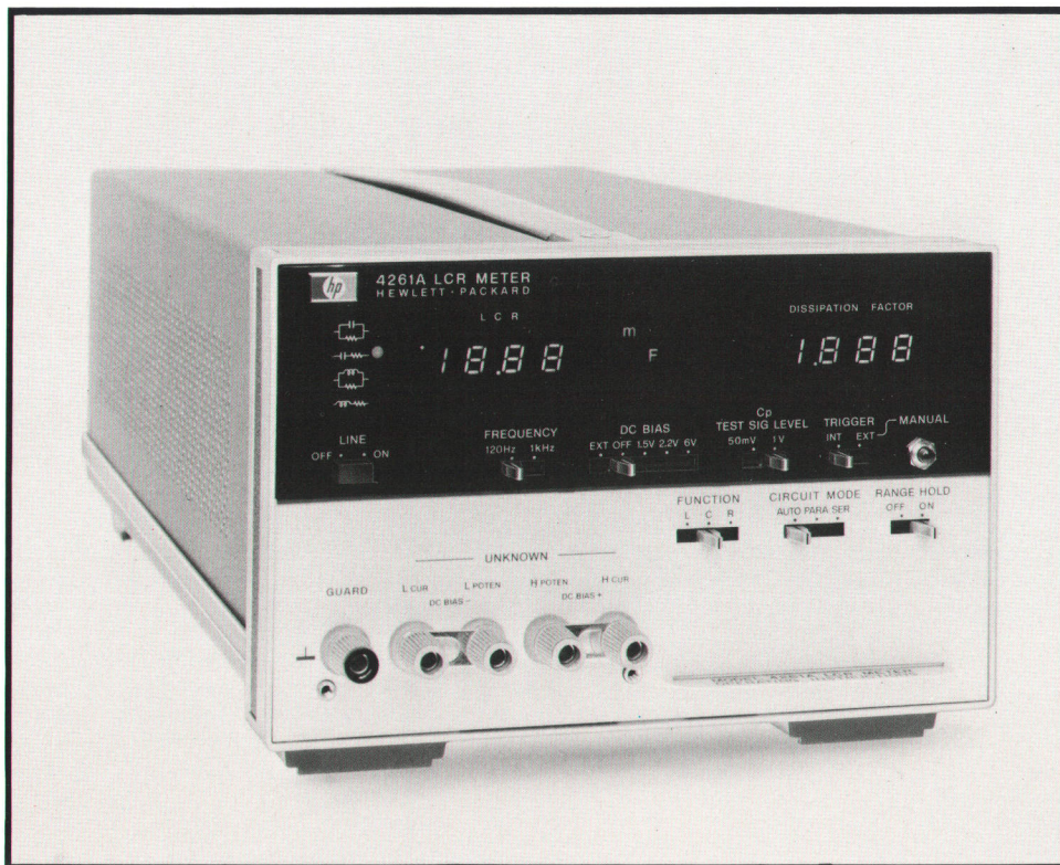
Fig. 1. Model 4261A LCR Meter makes fully automatic measurements of inductance, capacitance, resistance, and dissipation factor at 120 Hz or 1 kHz. It provides a choice of two test signal levels, three internal dc bias voltages, and two, three, or four-terminal measurement connections. HP Interface Bus (IEEE 488-1975) compatibility is optional.
